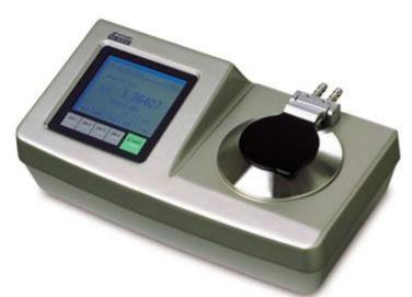
The digital refractometer RX-5000 has been developed to meet users' demands for fast, easy, accurate measurement. The RX-5000 measures samples for refractive index and Brix (%) (±0.00004 for nD, ±0.03% for Brix) in just four seconds. For most measurements, only two of the five operation keys are needed. In spite of the unit's compact size and light weight, performance has not been sacrificed. The RX-5000 is the desired refractometer for today's industrial demands.
